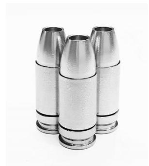
Liberty Ammunition's Ultra-Lights projectiles are copper monolithic with nickel plating and are turned on a precision CNC machine for consistency and accuracy. They are lightweight, extremely fast projectiles, with a large diameter deep hollow-point cavity.
