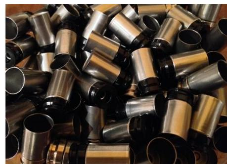
The proprietary nickel alloy stainless cylinder offers uniform wall thickness and a case capacity that is fractionally larger than a standard 9mm shell. Outside dimensions comply with SAAMI specifications. In addition, the case design incorporates a fractionally larger flash hole which helps eliminate back-face pressure, increases burn efficiency and is ideal for the new generation of environmentally friendly primers.
